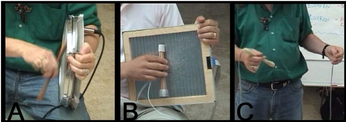
Figure 2: The three hardware controllers used to implement the Virtual *Bodhran*, the *Vodhran*. (A) The ddrum, (B) the Radio Baton, and (C) the Polhemus Fastrack.
